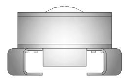
The Deck Edge Light (DEL) is designed to mark the deck's outer limits (perimeter circle) and complies with STANAG 1445 (NVG operations). For this purpose a dimming level of down to 0,05% can be achieved. It has a low and compact housing profile, which is made of massive seawater resistant aluminum for performance in rough marine environments.
